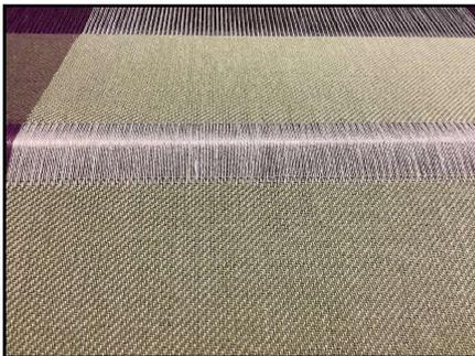
An extra piece of cloth which can be cut across so that the cloth roller can be unloaded before it becomes too heavy
