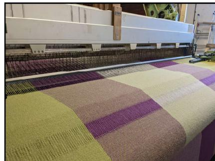
Heddles are wires that can raise the upper sheet of the warp
