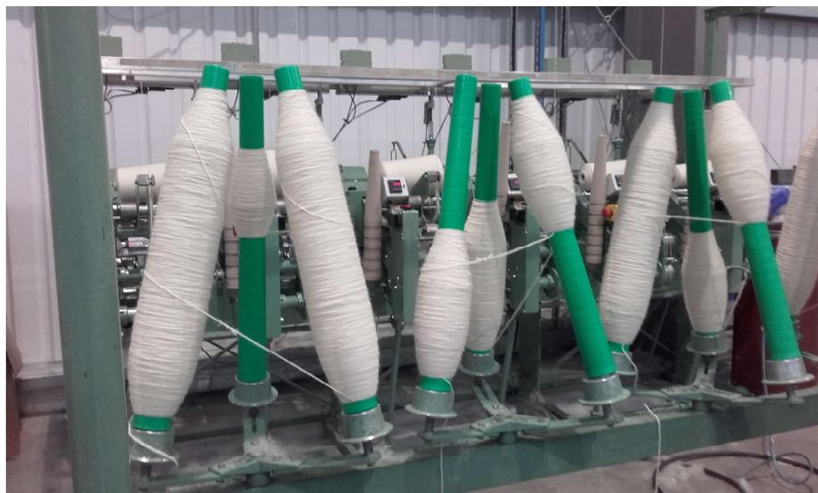
Checking rovings for faults
