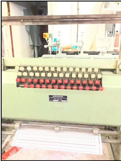
The machine that makes the holes that create the instructions on the loop
